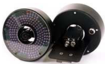
Figure 1.6: Array of infrared-emitting diodes mounted around a digital camera of a motion capture optical system with passive markers (BTS S.r.l motion capture system).
