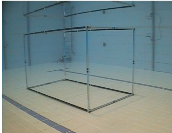
Figure 3.3: Grid employed for extrinsic calibration of the cameras.
