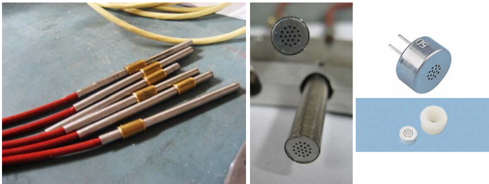
FIGURE 5.10: Close-up look of used microphones: assembled configuration, mounted configuration and original PCB capsule.
