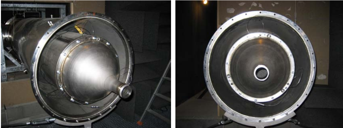
FIGURE 4.5: Closeup of jet exit during mounting and setup (terminal nozzle is absent).
