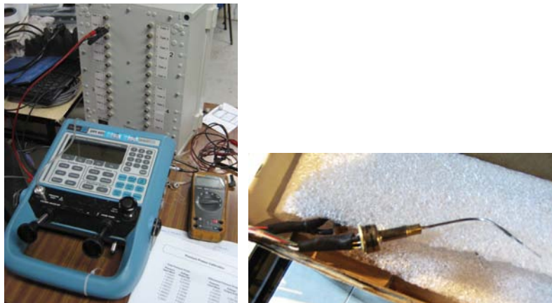
FIGURE 5.3: Probes calibration procedure: used instrumentation and pitot tube.
