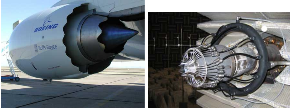
FIGURE 1.6: Example of chevrons and microjet systems for reducing jet noise.
