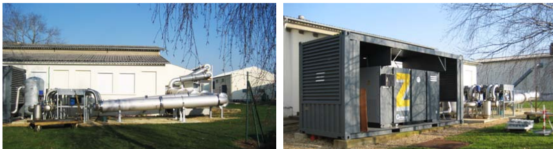
FIGURE 4.1: Exterior of the facility: subsonic wind tunnel “Bruit & Vent” and particular of the new installed hi-power compressor.
