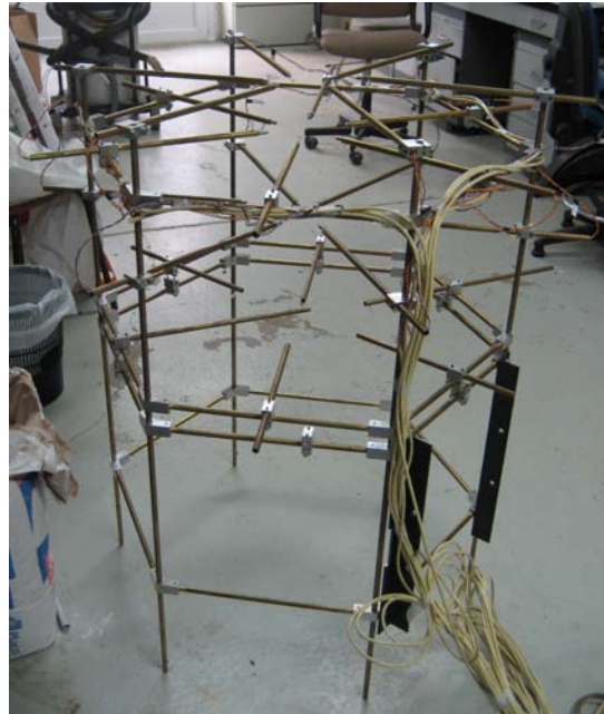
FIGURE 5.6: Near field antenna PAS setup and wiring operations.
