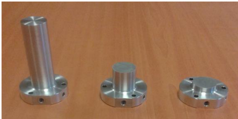
Figure 5.2: The exchangeable gas cells of different lengths (7.5 cm, 3.5 cm and 2 cm).
