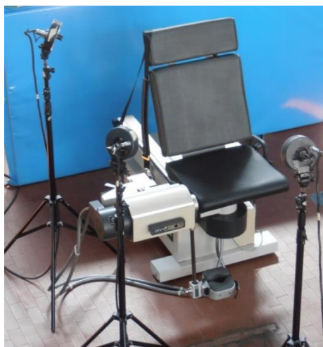
Fig.6.3: Optoelectronic system (only three cameras are shown).
