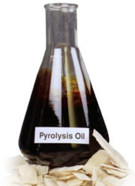
Figure 3: Bio-oil Produced from the Pyrolysis of Biomass (Lee et al., 2013).
