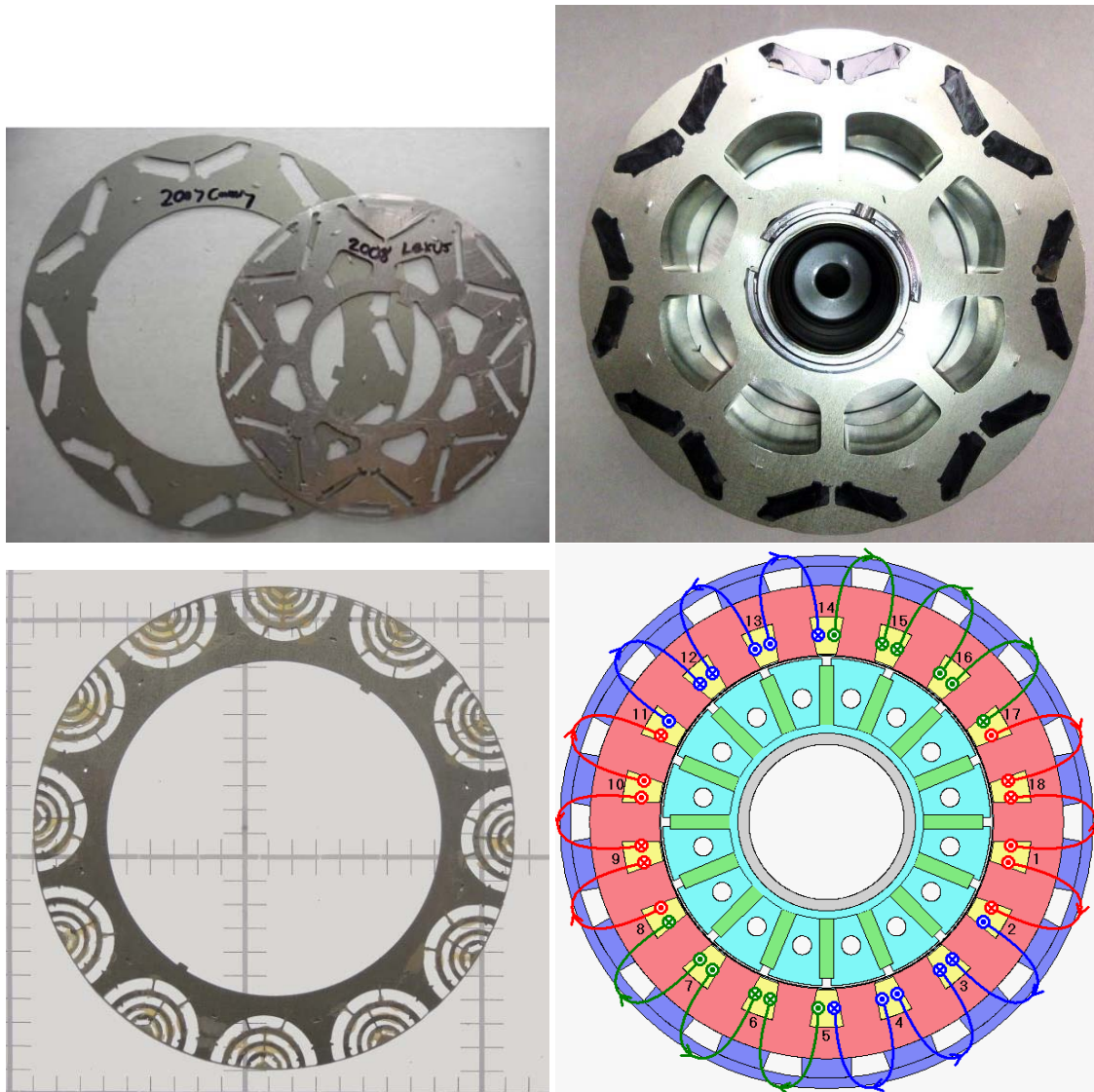
Figure 1.12: Examples of different rotor structures for actual automotive IPM motors.
