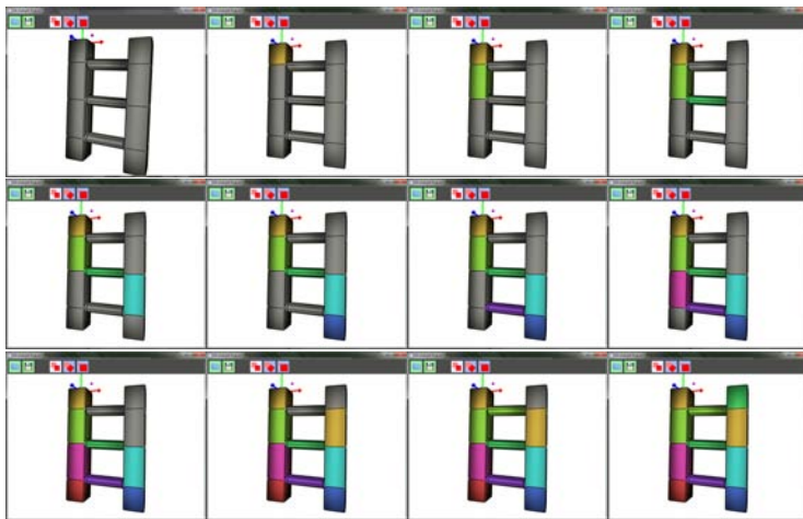
Figure 7.2: Skeleton recognition: mesh with loops (ladder)
