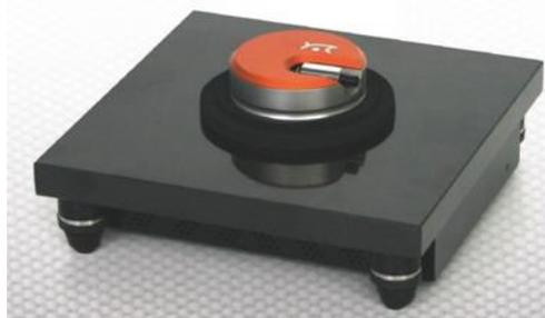
FIGURA 4.9 - PIANO D'APPOGGIO DEL STM *EASYSCAN*.
