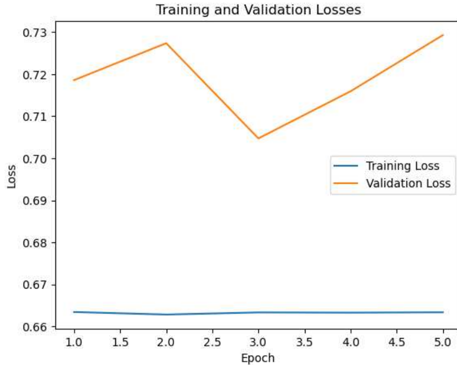
Figure 5.2: The plot of the training and validation loss for the DeepConvNet model. The training loss remains relatively stable across epochs, hovering around 0.665, suggesting that the model maintains consistent performance on the training data. However, the validation loss exhibits erratic fluctuations without showing a clear trend towards convergence. This inconsistency indicates potential overfitting to the training data, where the model performs well on the training set but struggles to generalize to unseen data, resulting in elevated validation loss. The training was stopped after a few epochs (5) due to the absence of improvement in validation loss. In fact, the validation loss begins to increase without showing any signs of improvement, as depicted on the plot.
