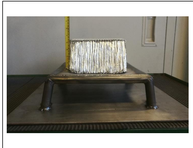
Figure 4: Attenuator after Impact
