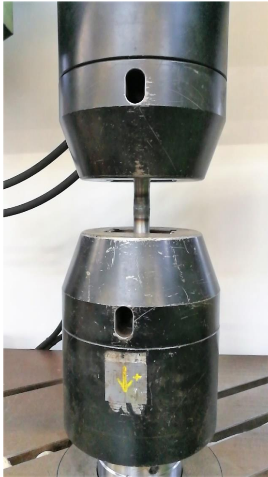
FIG. 3: View of the test welded tube in the jaws of the tensile test machine.
