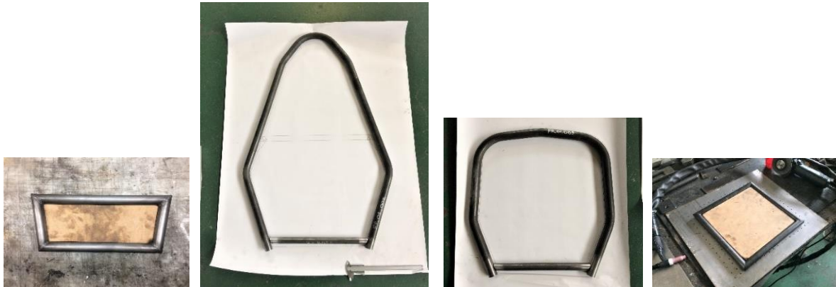
Figura 4.9: Trapezio posteriore; main hoop section; front hoop section; front bulkhead section.
