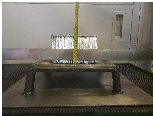
Fig.16: Measuring method of AIP deflection
