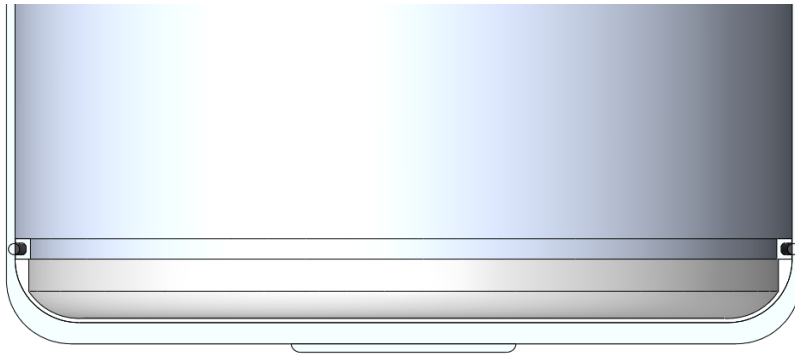
Figure 3.9: Teflon separation element bottom end configuration where the design of the disk follows the curvature of the tank.
