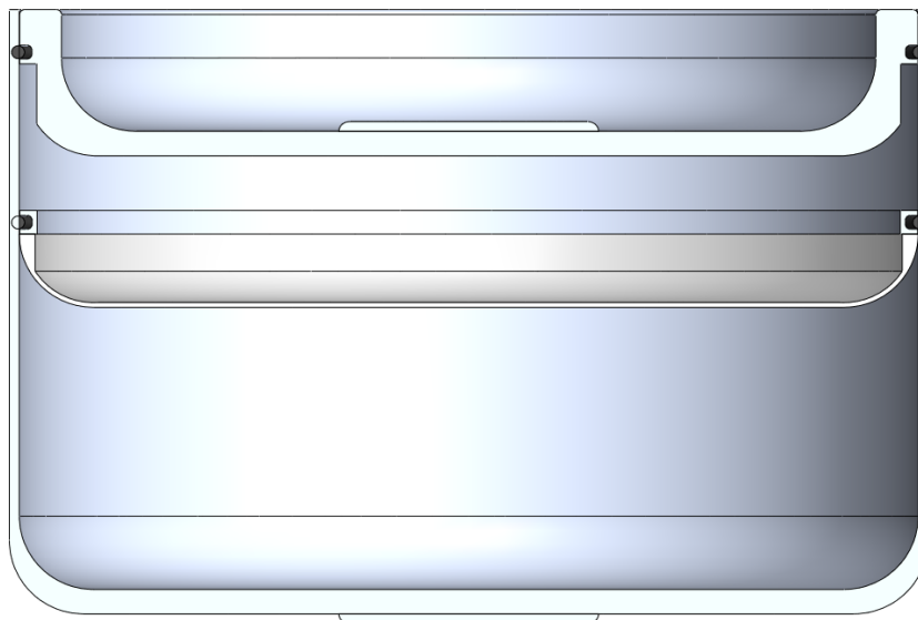
Figure 3.14: Sectional view of the final design for the propellant tank.
