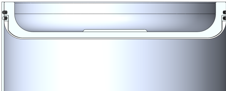
Figure 3.10: Teflon separation element top end configuration where the design of the cap follows the curvature of the piston.
