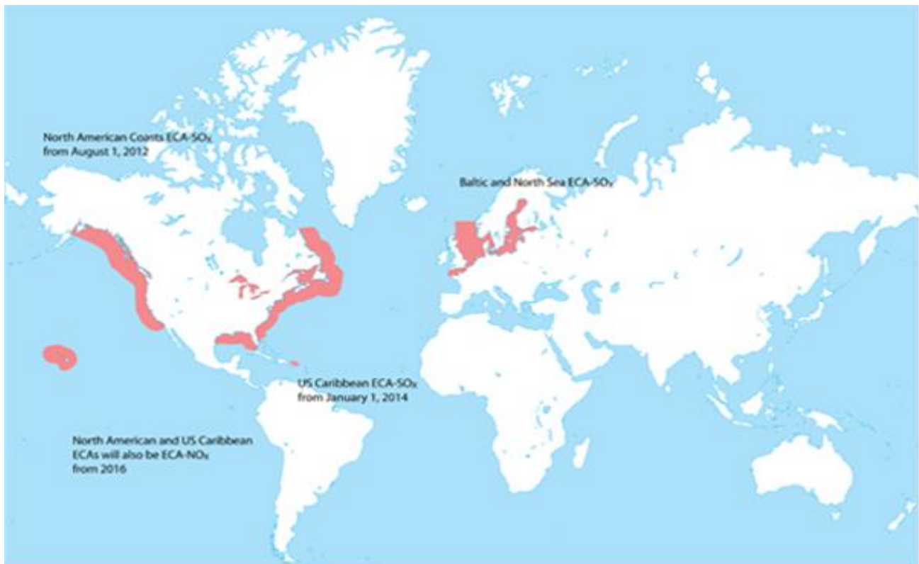
Figure 1.8 The Emission Controlled Area, where Tier III will be applied starting from 2016
