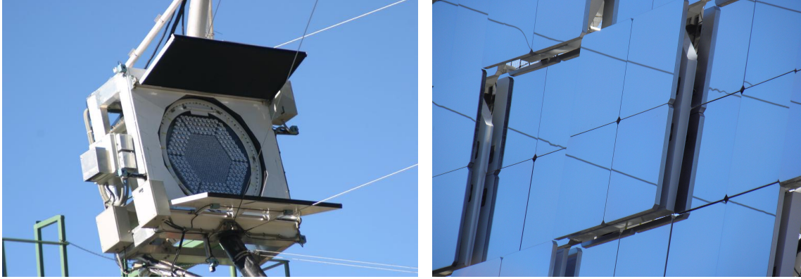
Figure 3.12: Camera and mirror images of MAGIC telescopes. Left: Foreview of the camera. Right: Individual segments of the mirror.
