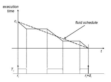
Figure 4.1: Task fluid diagram
