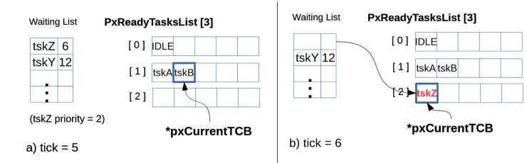
Figure 2.6: preemptive context switch - a) )description of the Waiting List and Ready List at tick=26; b) when tick=27, tskA moves in the Ready List and goes in Running state
