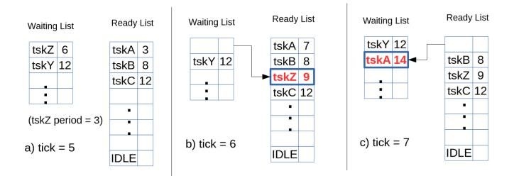
Figure 3.4: a) tskA is the running task, its deadline is at tick = 6; b) tick mechanism wakes tskZ removing it from Waiting List and adding it to Ready List, in the right position according to its new deadline:  $Z_{deadline} = tick + Z_{period} = 9$ ; c) tskA ends its execution and is moved to the Waiting List. tskB now is on the head of the Ready List.
