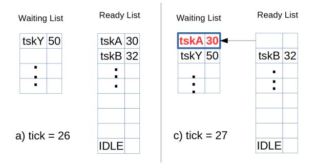
Figure 3.7: Collaborative example- a)description of the Waiting List and Ready List at tick=26 b) when tick=27, tskA moves in the Waiting List and tskB became the executing task
