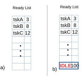
Figure 3.5: a) tskA, tskB and tskC are created before the sceduler is started; b) vTaskStartScheduler() method is called, the real time kernel tick processing starts and the IDLE task is added at the last position of the Rady List. It will execute only when no other tasks are in ready state.
