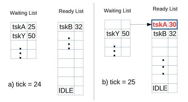
Figure 3.6: a) tskA will be awaken at the next tick. tskB has the nearest deadline among the tasks in ReadyList, so it's in the head position. IDLE is the task with the farest deadline. b) After the tick interrupt happened, tskA moves to the Ready List:  $tskA_{deadline} = currentTick + tskA_{period} = 25 + 5 = 30$
