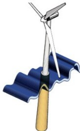
Figure 8. Sketch of ballast stabilized floating wind turbine [26]
