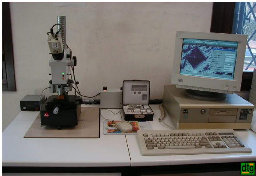
**Fig 4.8: Microdurometro**
