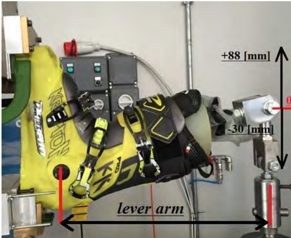
Figure 6.16 The Neutral position ( F=0 ), the boundary values of the maximum flexion (+88 [mm]) and maximum extension (-30 [mm]);
