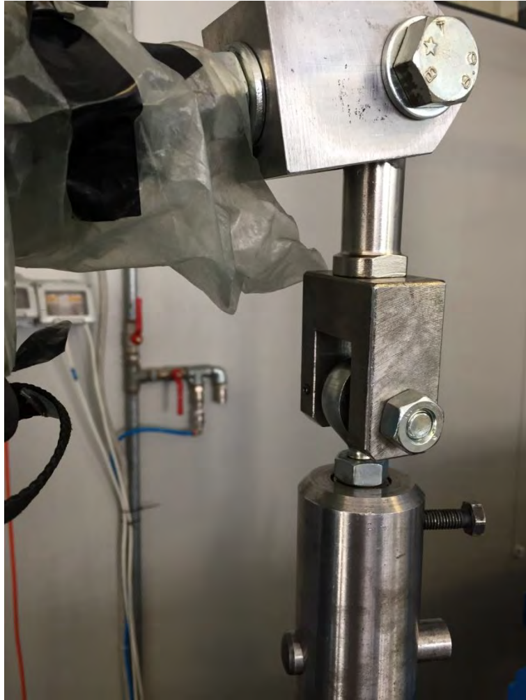
Figure 6.14 The other extremity of the rod is jointed with the prosthetic leg by another junction.
