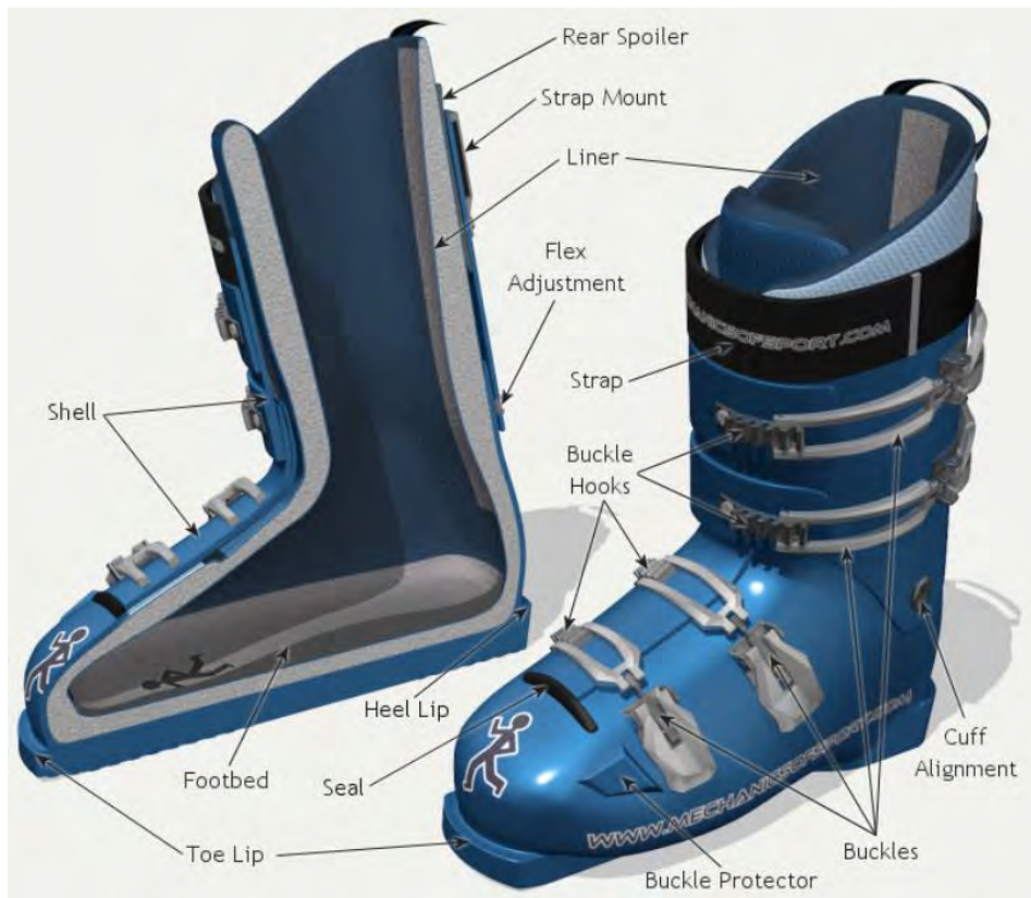
Figure 1.8 Parts of a ski boot.
