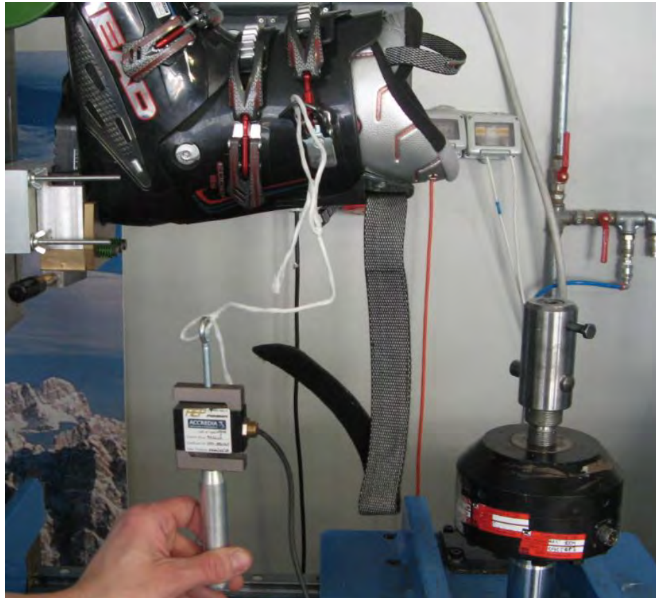
Figure 6.12 The manual load cell employed in measuring of the closing force of single buckle.
