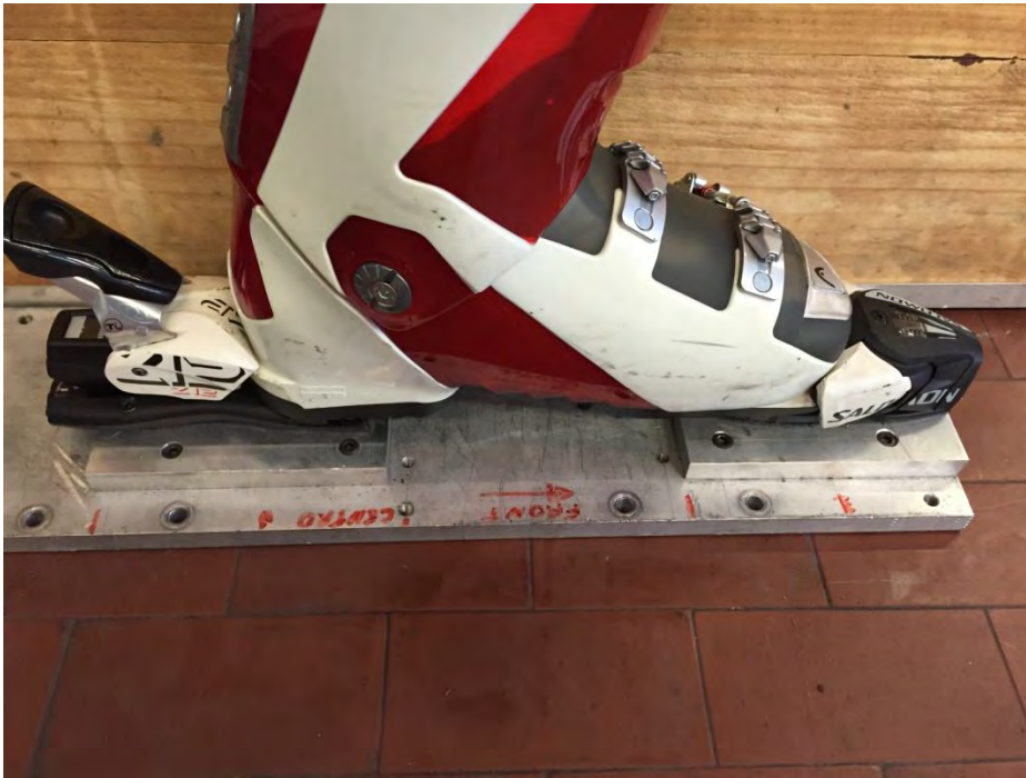
Figure 6.5 The "Ski binding" employed in Padua's axial work bench
