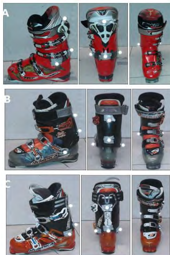
Figure 5.7 (A)Tecnica, Phnx 100; (B) Nordica, Hell and Back; (C) Nordica, Firearrow; (D) Dalbello, Krypton. Illustration of the application points of the markers.
