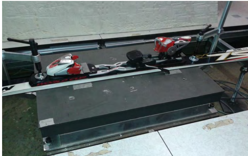
Figure 5.8 The ski fixed on the dynamometric platform
