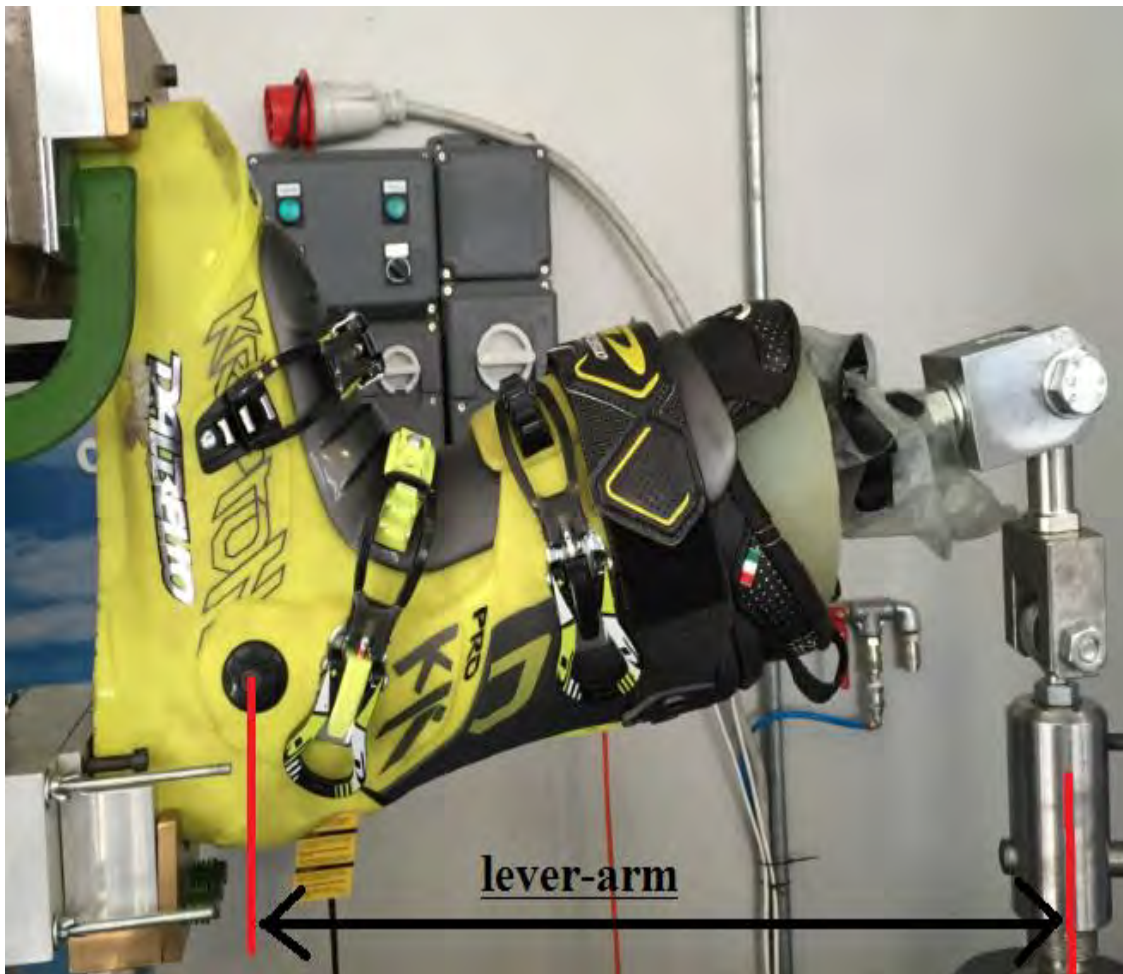
Figure 6.15 The lever arm between the centre of the axial machine and the hinge of the ski boot.
