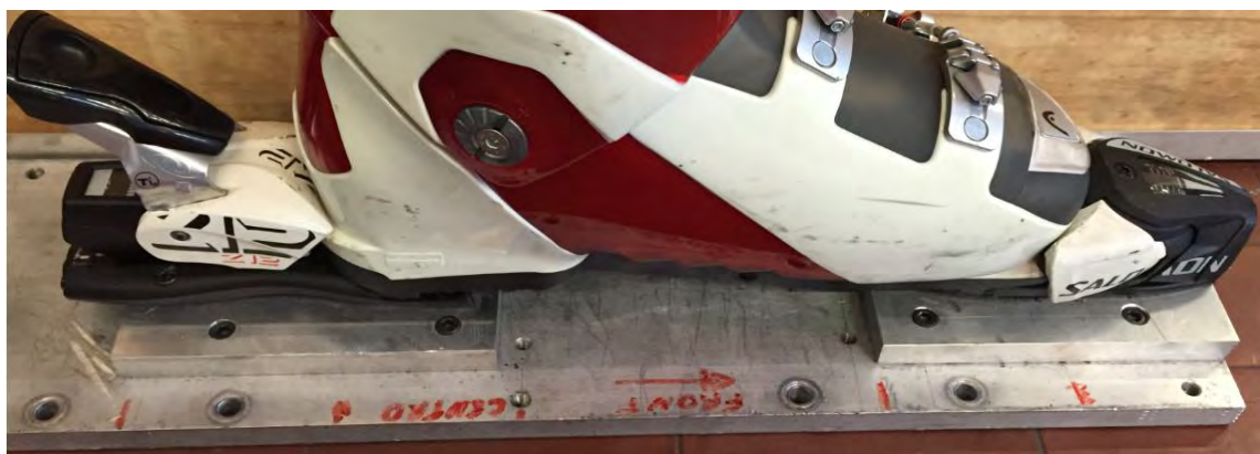
Figure 4.27 The ski binding employed in the UPF and in UPT.
