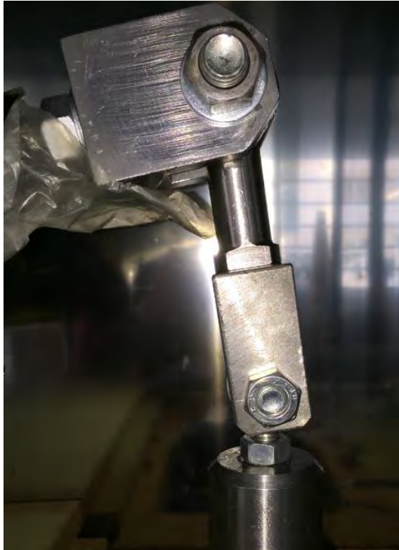
Figure 4.35 The connecting rod with the two joint: one with the prosthesis (above) and the second with the actuator (below).
