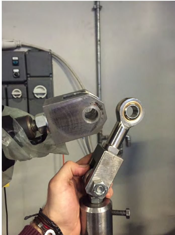
Figure 6.13 In the part below of the figure the extremity of the axial machine that is jointed with the rod through a junction.
