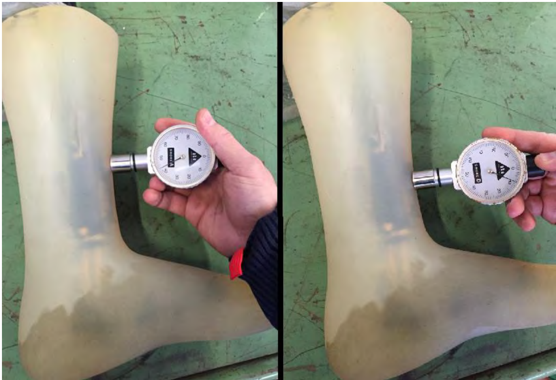
Figure 4.2 From the left to the right: the hardness measured with a Durometro type A and with a Durometro type D.
