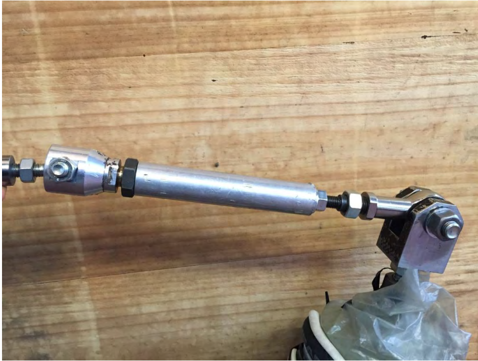
Figure 6.7 The connecting rod, which is attached to the hydraulic actuator (the extremity on the left) and to the prosthetic leg (the extremity on the right).
