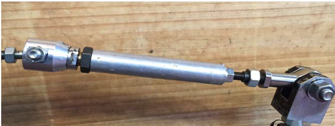
Figure 4.28 The connecting rod and its spherical joints.
