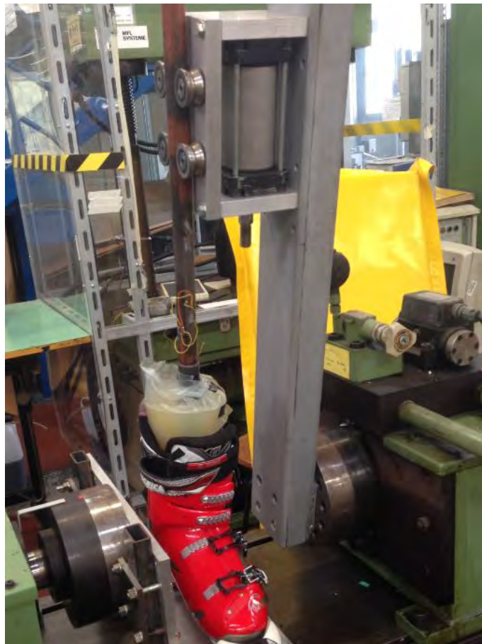
Figure 4.24 Mechanical arm connects with motor-spindle of torsion machine
