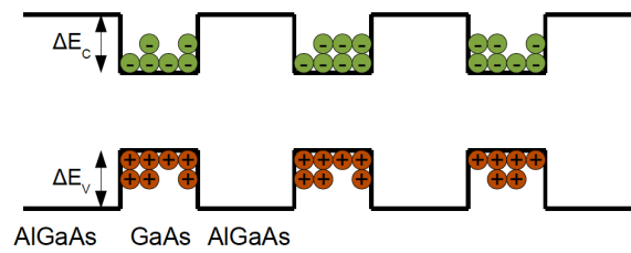
Figure 2.14: The structure of a MQW formed by layers of AlGaAs and GaAs
