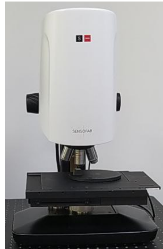
(b) Profilometer used for wear measurements.
