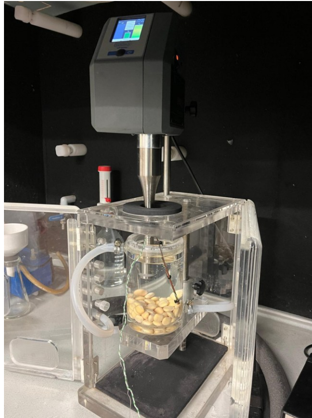
Fig 3.4: Setup and application of HPU on lupine seeds
