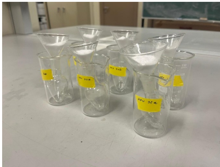
Fig 3.7: Filtration of organic phase for alkaloids extraction
