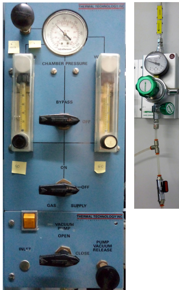
Fig 4.9 Controlled atmosphere system during sintering in the furnace;
