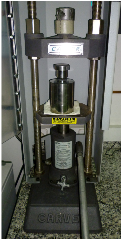
Fig. 4.4 (a) Uniaxial Carver C press, with mould of stainless steel; (b) phase of weighting of ZrB_2 before mixing;
