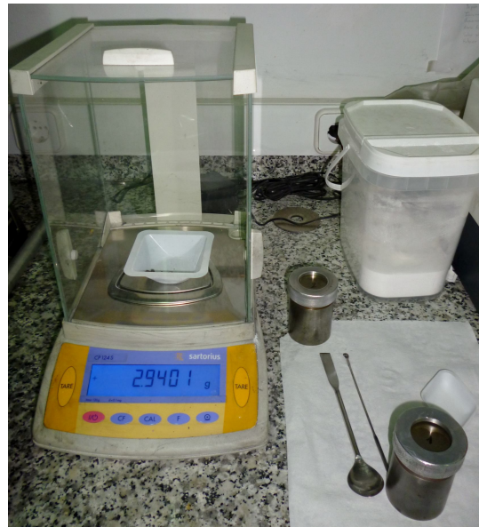
Fig. 4.4 (a) Uniaxial Carver C press, with mould of stainless steel; (b) phase of weighting of ZrB_2 before mixing;
