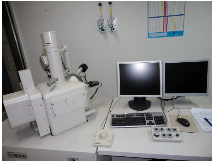
Fig. 5.4 A typical SEM instrument, showing the electron column, sample chamber, EDS detector, electronics console, and visual display monitors;
