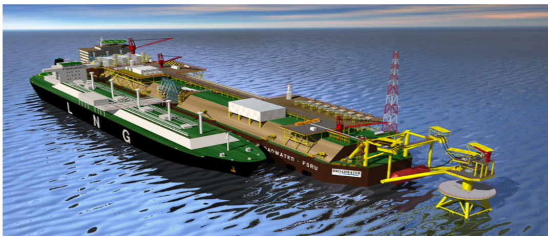
Figura 2.5 – Floating Storage and Regasification Units fissa (FSRUs).
