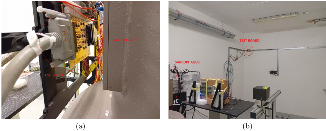
Figure 3.17: OP07 ELDRS test board placement inside the CC60 irradiation room. (a) High dose rate irradiation: the board is placed close to the sarcophagus aperture. (b) Low dose rate irradiation: the board is placed in the peripheral wall in front of the sarcophagus aperture.
