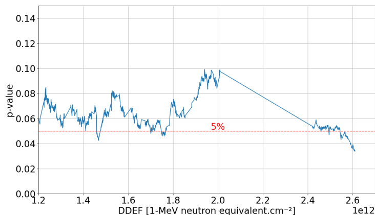
Figure 4.9: Profile of the p-value associated to the ANOVA test as a function of the displacement damage equivalent fluence concerning the input voltage degradation of the operational amplifier LM358AD.
