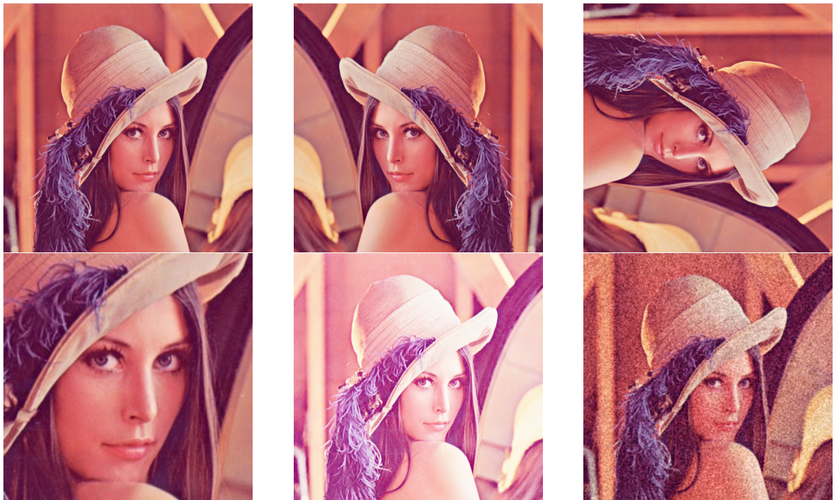
Figure 1.4: Common data augmentation transformation applied to an image. (Top row) original image, mirroring and rotation. (Bottom row) cropping, brightness variation and noise adding
