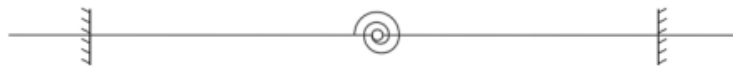
Schematization of real behavior double leaf Bascule Bridge with active mid-span shear locks
