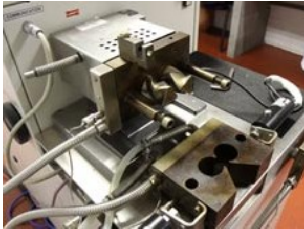
Figure 23 Internal mixer for blending (BRABENDER).
