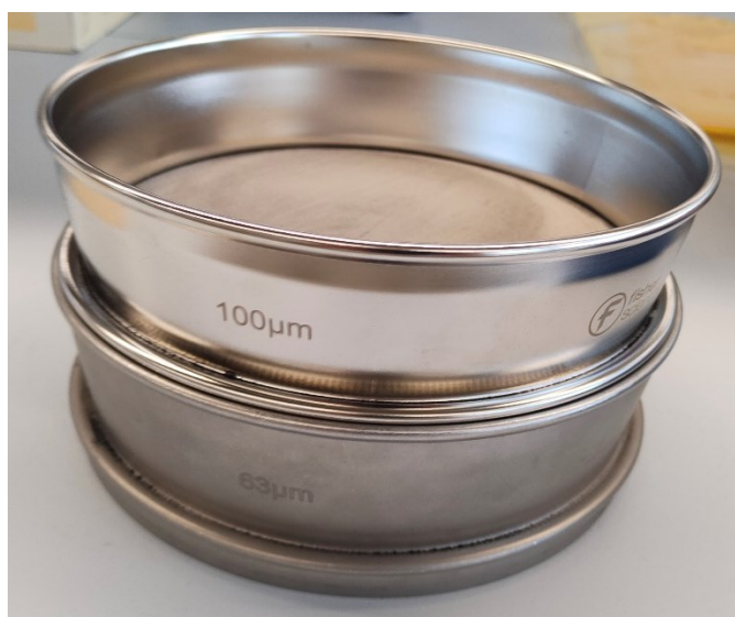
Figure 19 Sifters for 63 \mu\text{m} and 100 \mu\text{m} sieving.
