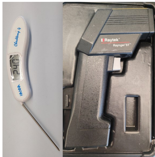
Figure 21 On the left, contact digital thermometer (HANNA). On the right, laser digital thermometer (Raytek).
