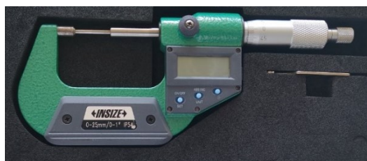
Figure 29 INSIZE Micrometer for thickness measurements.
