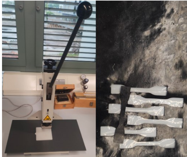
Figure 26 Stamping machine and NR/GTRD sample.
