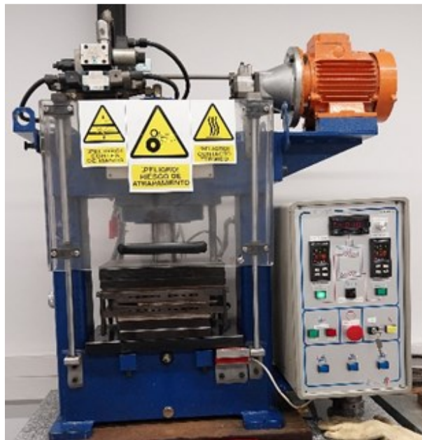
Figure 25 Hot press for molding and vulcanization.
