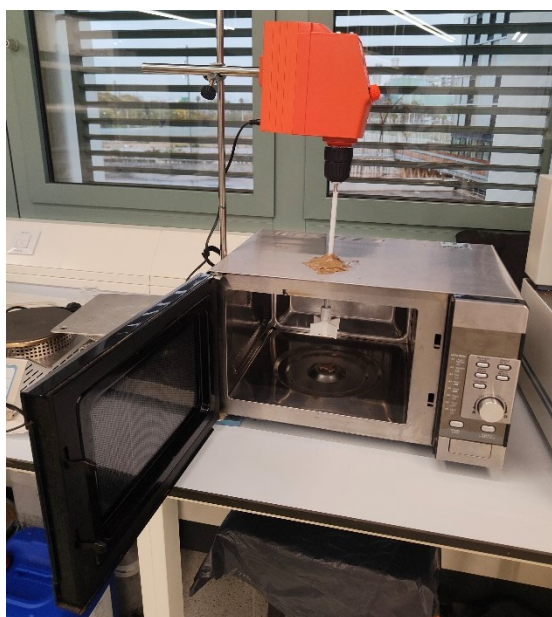
Figure 20 Microwave apparatus for devulcanization.
