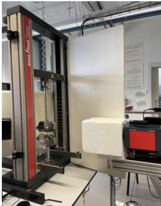
Figure 34 On the left the tensile testing machine. On the right the IR camera.
