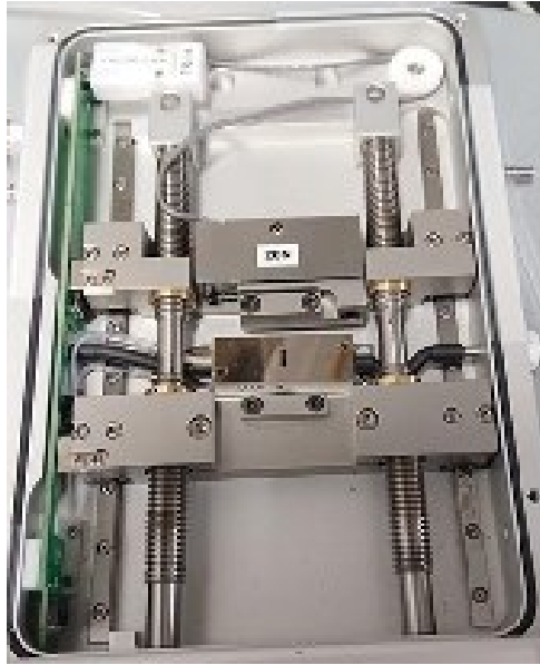
Figure 28 Stretcher - TST350 for uniaxial tensile tests.
