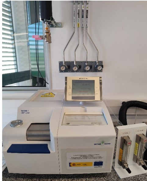
Figure 32 Machine and gas regulation system for TGA.
